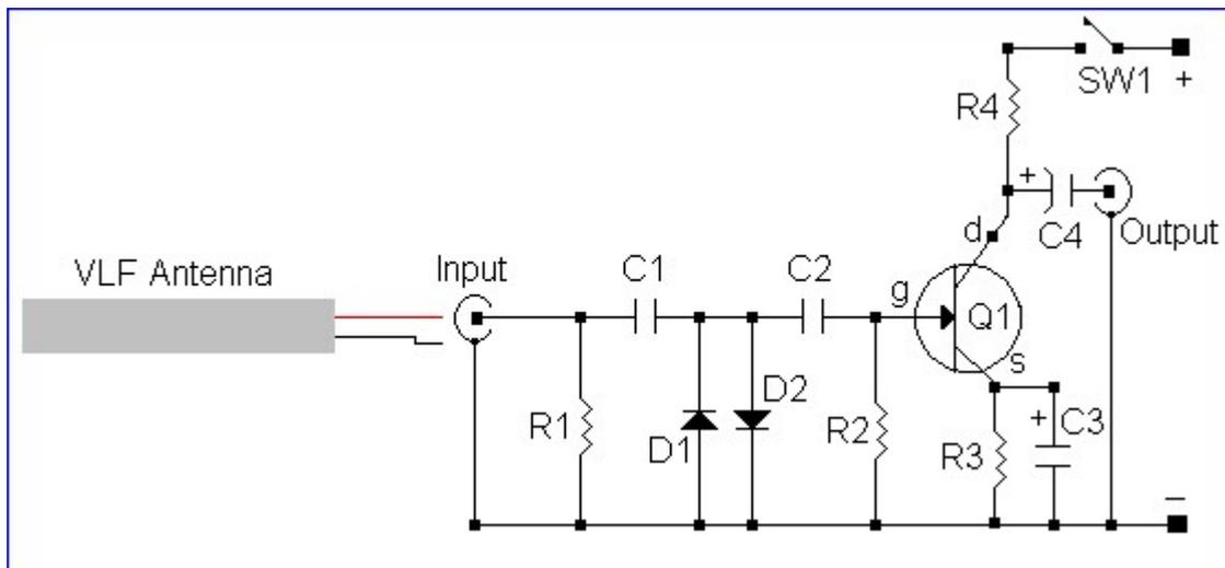
This FET preamp makes a great unit to place ahead of a tape recorder or portable audio amplifier. It adds very little hiss noise unlike bi-polar transistors do.
