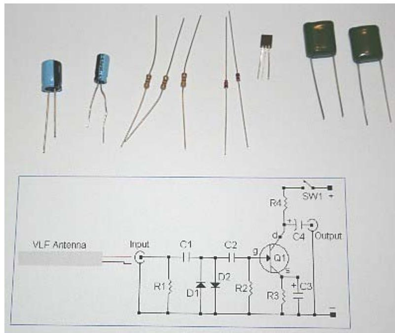
You can place a capacitor across R1 for a wide-band general tuned circuit. You can remove R1 for a sharply tuned circuit.
