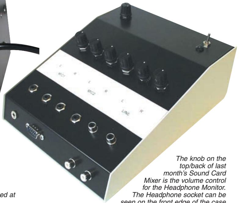
The knob on the top/back of last month's Sound Card Mixer is the volume control for the Headphone Monitor. The Headphone socket can be seen on the front edge of the case
