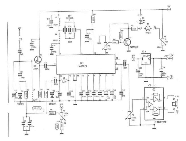
Circuit diagram 1 SW receiver for 4.5 - 11 MHz
