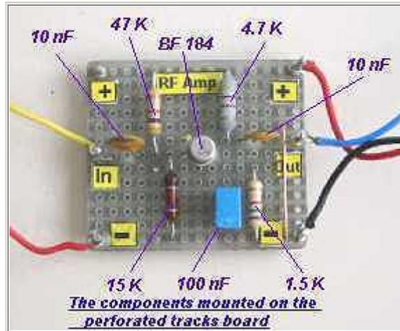
This 'AM-FM Radio Frequency Amplifier' is built with only a few components; which makes the project simple and direct. There are no electrolytic capacitors and the three capacitors used can be ceramic or mylar. You can employ 1/4 watt resistors or even 1/2 watt resistors which are easier to manage.
