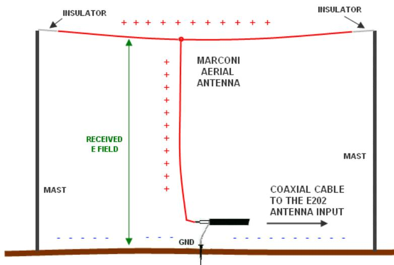
The dimensions are not critical because the antenna is not resonant: 3 meters vertical and 6 meters horizontal are sufficient to provide a large increase in efficiency compared to a 75 cm stylus; especially in the reception of frequencies below 100 Hz.
