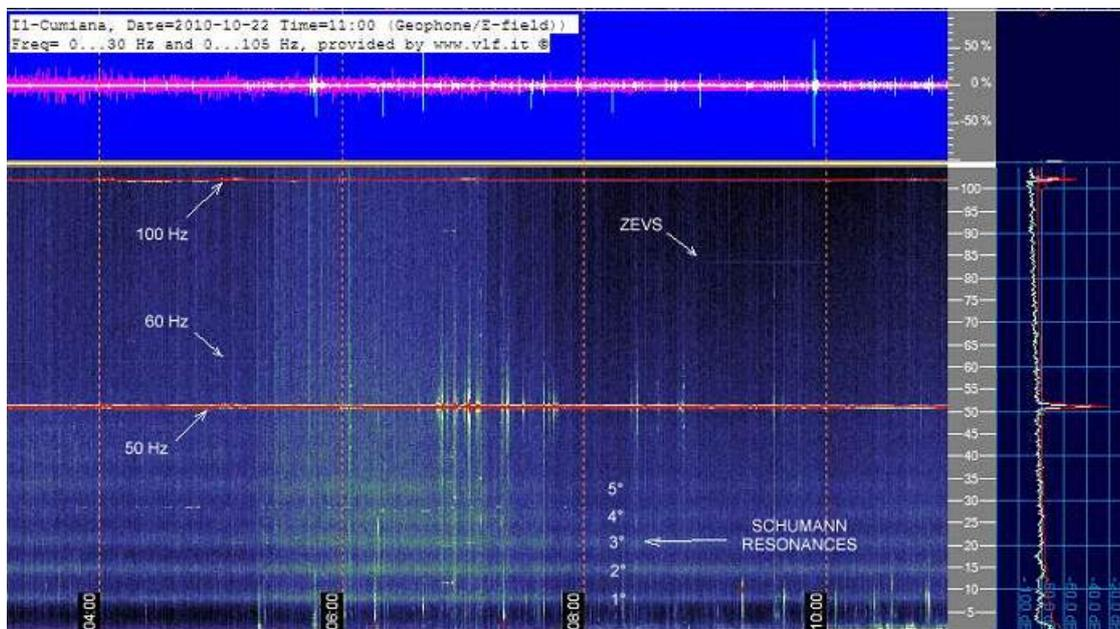
In the spectrogram above, developed with SpectrumLab and obtained on a received signal with a Marconi wire antenna, are visible: the Schumann resonances, a 82 Hz Zevs signal from a Russian submarine broadcast network, 50 Hz network, the first harmonic at 100 Hz and the weak 60 Hz signal of American power grid.
