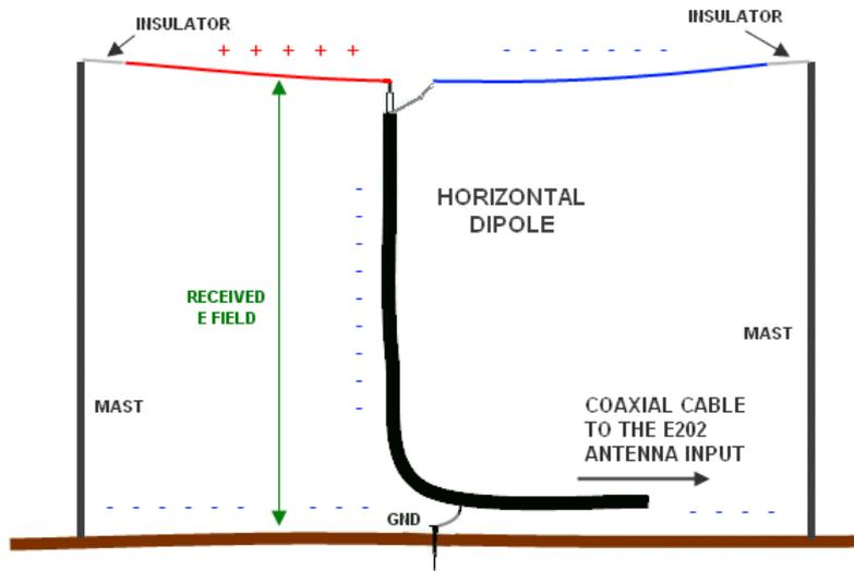
The figure above shows how a horizontal dipole behaves at VLF frequencies. The receiver is not differential but referred to ground, so the received component will always be the vertical one, even with the antenna placed horizontally. This is because the antenna is much shorter than the signal wavelength and therefore does not behave as an antenna but as a field probe. It detects the vertical voltage between two points: the ground and the antenna.
