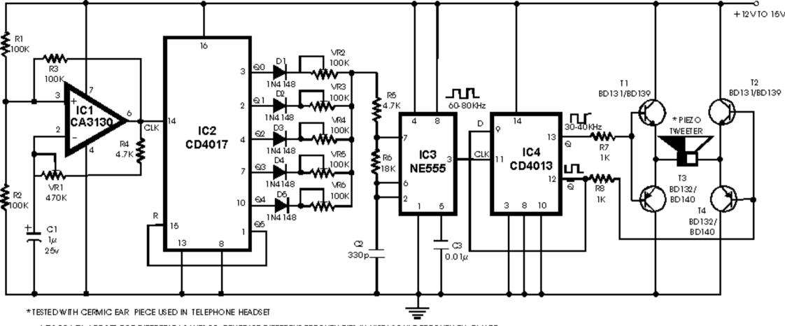
VR1 TO VR6 ARE SET FOR DIFFERENT VALUES TO GENERATE DIFFERENT FREQUENCIES IN ULTRASONIC FREQUENCY. RANGE
