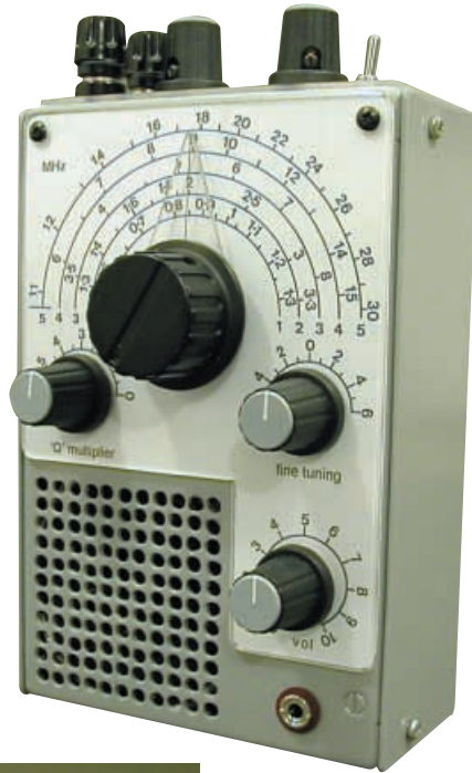
Fig.10 (above right). Top and front panel control dials reproduced half size. The completed Receiver is shown top left
