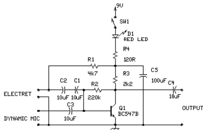
Simple microphone preamplifier
