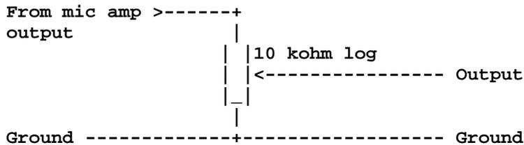
This circuit allows adjusting the output level between zero and the maximum microphone preamplifier amplification.
