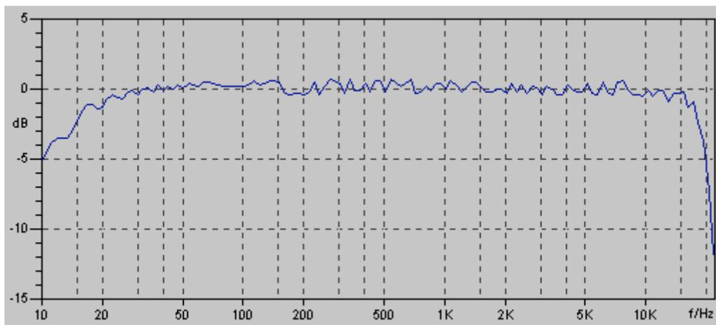
The bass frequency attenuation is caused by the microphone preamplifier circuit. The high end attenuation is caused by Sound Blaster 16 card. As seen in the measured performance, the microphone preamplifier is suitable for speaker measurements made using suitable measurement software and sound card. Using this preamplifier connected to line level input the problems caused by poor microphone preamplifier in many sound cards can be avoided.
