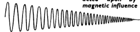
Fig. 3. Diminishing alternating voltage set up by precession frequencies from the detector coils
