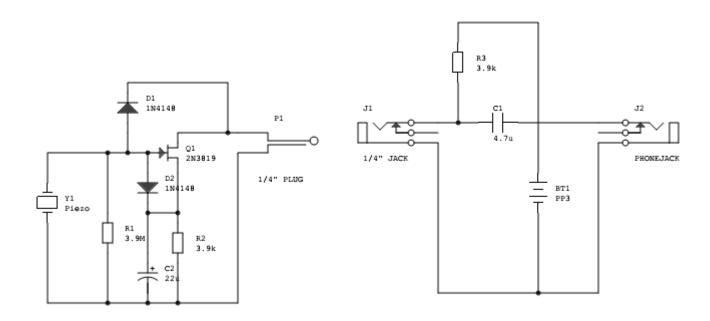
By using a separate box for the battery and load resistor the circuit is automatically powered when you plug in the piezo device. By keeping the FET close to the piezo disk you maximize signal levels and reduce the extent of the high impedance part of the circuit, which has a tendency to pick up hum. You also raise the signal level on the interconnecting cable run, which also helps to improve the system signal to noise ratio.
