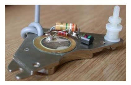
My original version of this (no diodes, C2 and slightly different source resistor) I glue the contact mic using epoxy resin to the back of the actuator magnet of an old hard disk. This is a nice strong magnet, and since many resonant structures are steel you get an instant easy good contact with the object.
