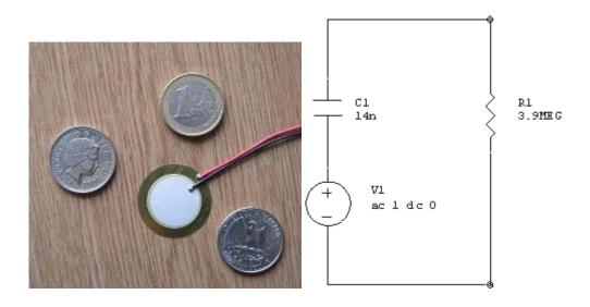
A piezo element can be thought of as a sound-dependent voltage source in series with a large capacitance of about 15nF.
