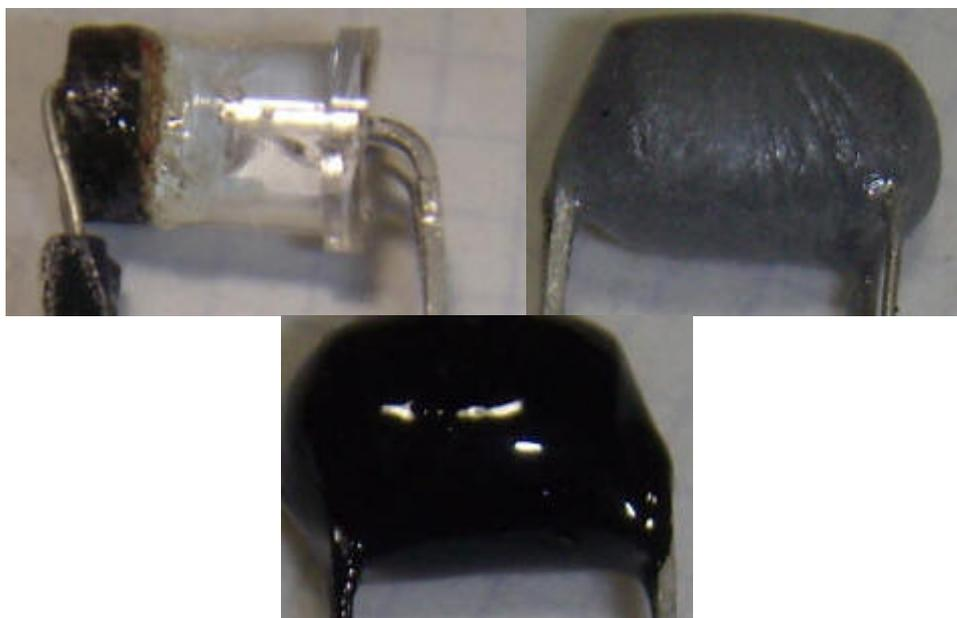
The AGC range is over 60 dB and the maximum gain is set by the 22 megohm across the photocell. Combined with the dynamic range of the sound recorder, the total range will extend from a whisper to a roar. The resistor in series with the LED sets the sensitivity of the AGC and that value may be increased if the loop is unstable, especially if the LED is a high-intensity type.
