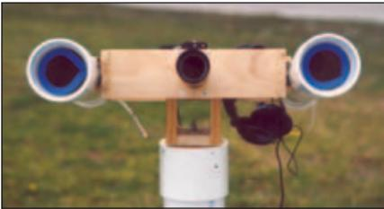
■ FIGURE 3. Front view of the microphone tubes showing the plastic foam inserts (blue) used as sound dampening material.
