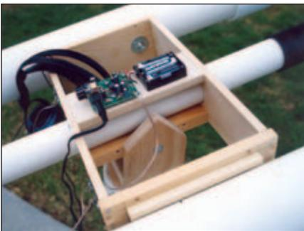
■ FIGURE 4. Placement of the battery holder for three AA batteries and of the Velleman "Super Stereo Ear" printed circuit board is visible, along with a close-up look at the altazimuth mount construction.
