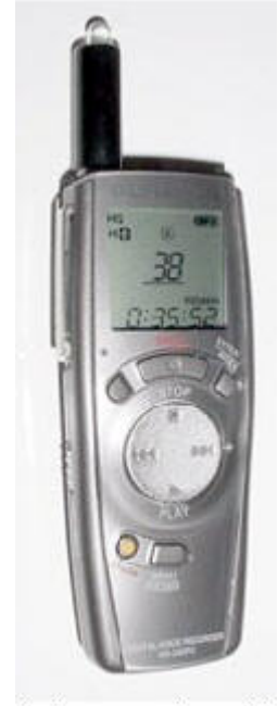
Audio recorder with detector mounted in microphone jack
