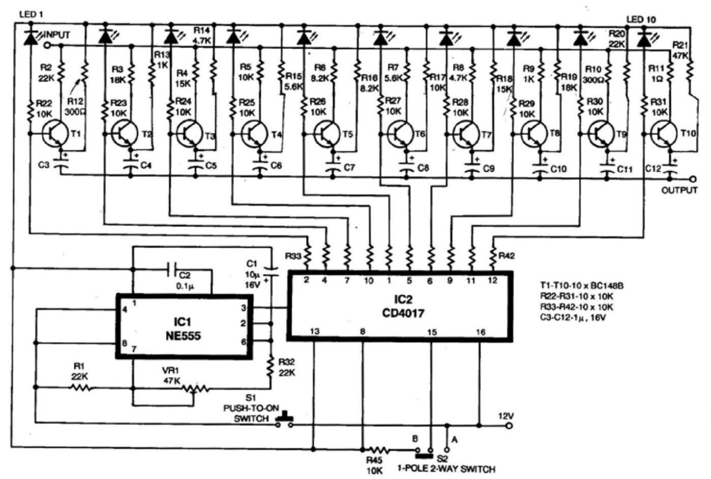
of the amplifier. This can be done with the help of decade counter IC 4017 and some transistors.
