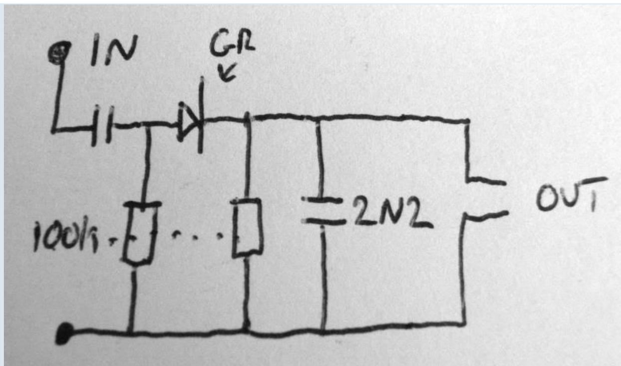
Left to right: Antenna, short wire with loop, 1n capacitor, loaded to ground at 100k ohms, Germanium diode, again loaded to earth at 100k ohms, then a 2n2 capacitor (made up with two caps in my circuit)
