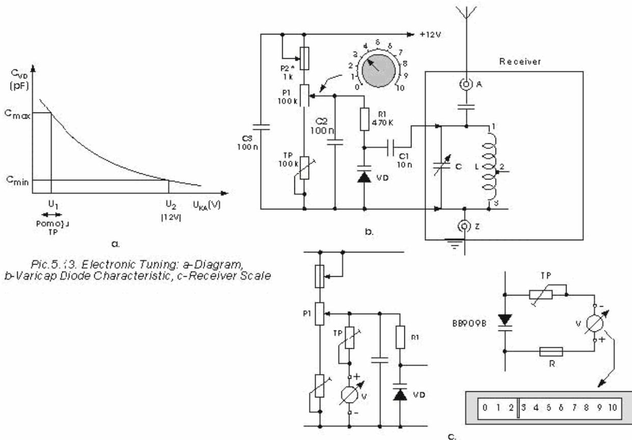
Fig. 5.13. Electronic Tuning: a-Diagram, b-Varicap Diode Characteristic, c-Receiver Scale
