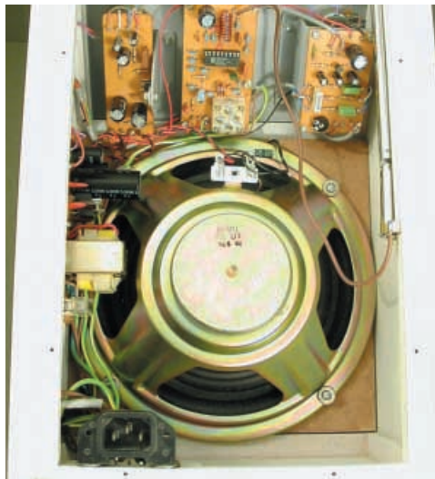
The Bass speaker and p.c.b.s mounted inside the wooden case. The h.f. speaker is glued to the back of the speaker grille.
