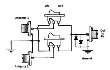
The circuit that is shown is extremely simple and it works in such way that you can connect an antenna or other and also both (it is single question of experiencing) with the extra attaché that in position (OFF) of both switch, the antennas are connected to ground and at the same time they disconnect the receiver achieving the wanted security.
