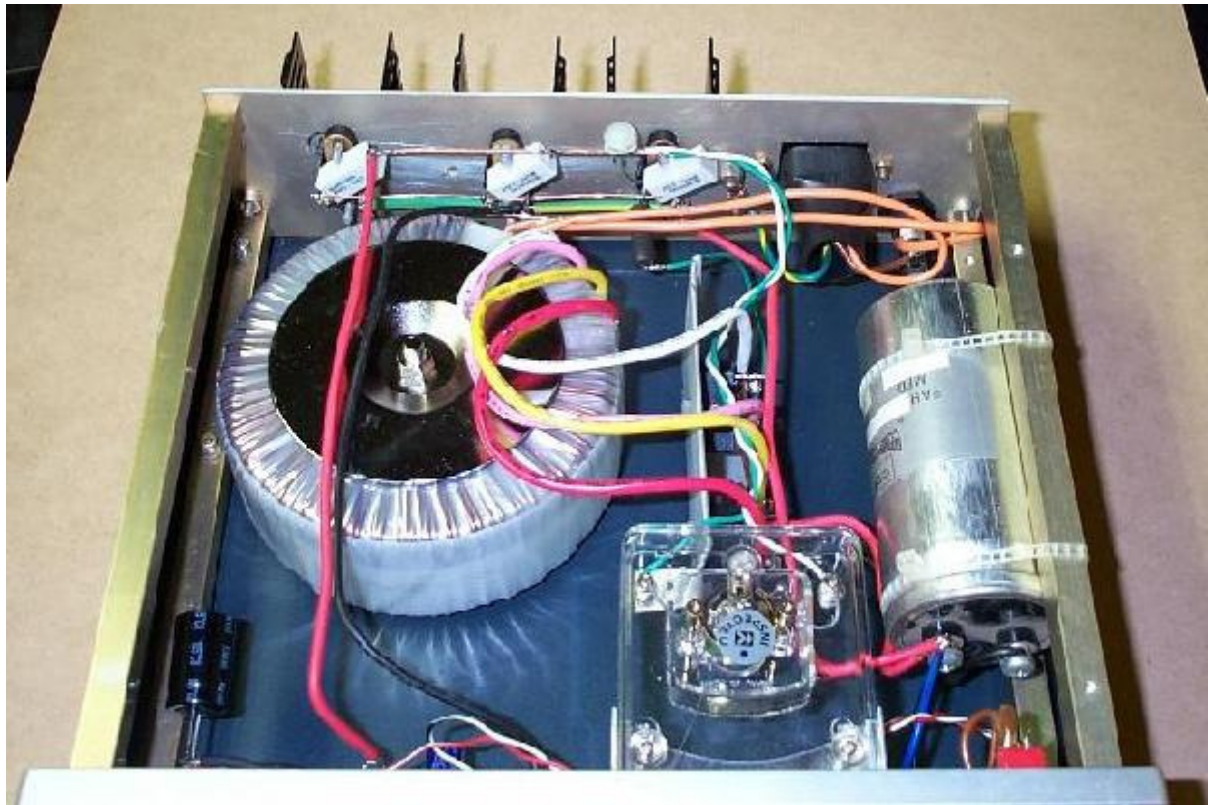
Figure 4 - Prototype Supply (Rear Panel Inside View) - 10A Version
