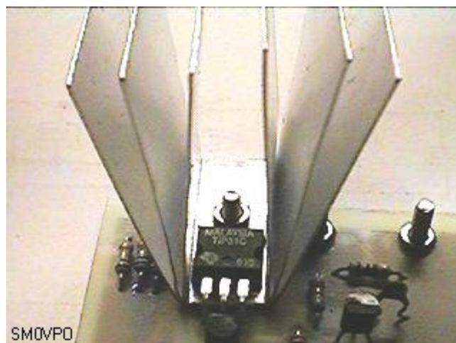
The heatsink shown above is three pieces of thin aluminium sheet, 11cm x 3cm drilled with a 3mm hole dead centre. These are bolted between the PCB and the TIP31 transistor before any other components are mounted on the board. The fins can now be bent up to form six fins, each 5cm x 3cm or a total surface area of 180cm square. This is a little bigger than the calculation, but to over-engineer is not a fault (at least, not in my opinion). Here is the completed project.
