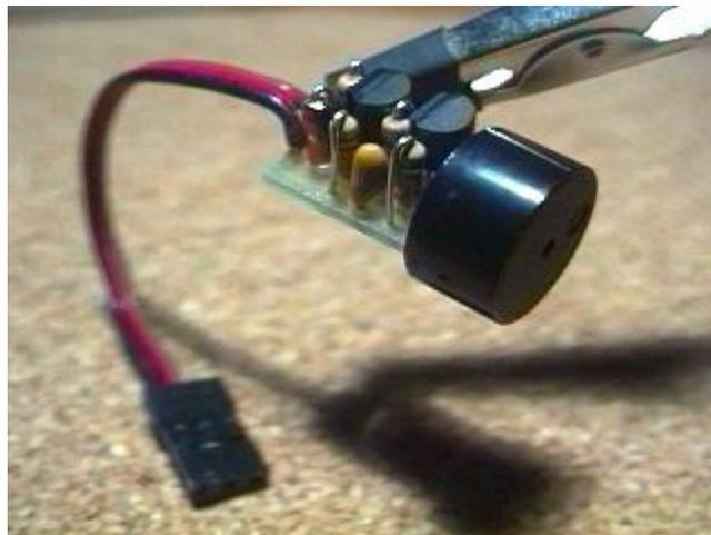
Radio Shack parts: Here again, you can use smaller rated resistors if you can get them--1/8 watt or less is fine. Tantalum capacitors are physically smaller, but any composition will work.
