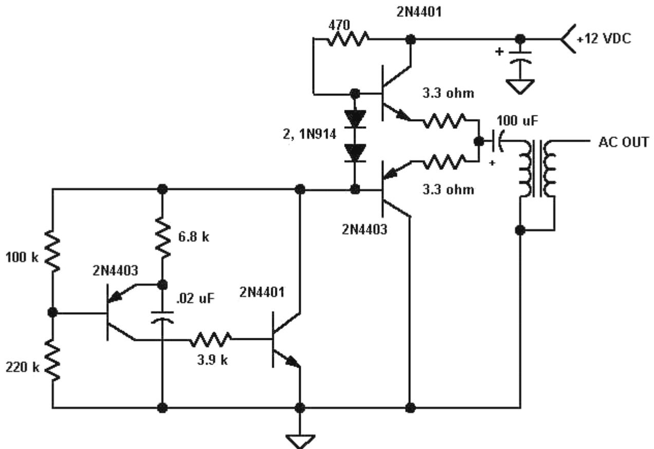
The transformer may be an audio type connected for step-up or step-down depending upon the desired output voltage. An old tube radio output transformer with the speaker winding connected to the circuit gave about 250 VRMS.
