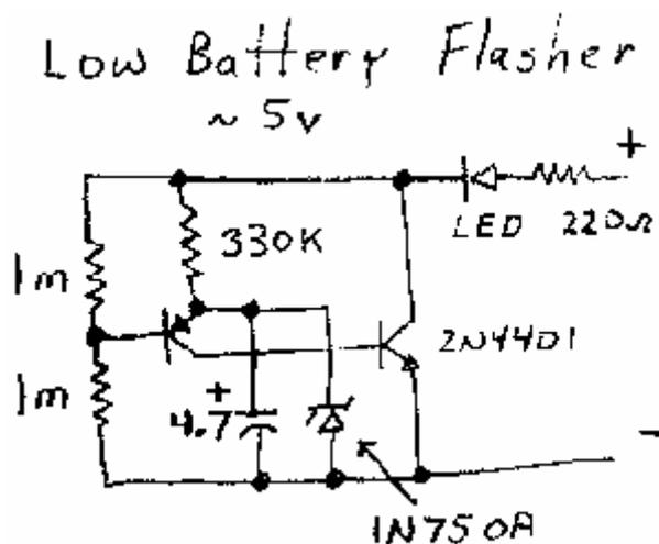
The zener is a "4.7 volt" type but in this circuit it is operating at a very low current and is limiting the emitter voltage to about 2.5 volts. Some experimentation may be necessary if another zener series is used.
