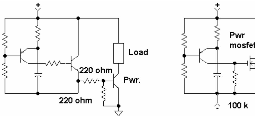
**Figure 2: Some typical flasher connections.**
