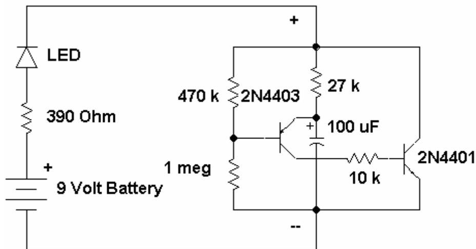
**Figure 1: Two-transistor lamp flasher.**
