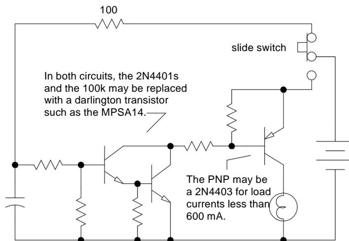
Circuit construction is not critical and point-to-point wiring on a small piece of perf-board is fine.
