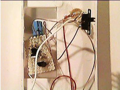
Some battery-powered devices have very little space to hide the circuit so a little planning can save much rework. Notice how the capacitor was moved to lower the profile for this dollhouse installation.
