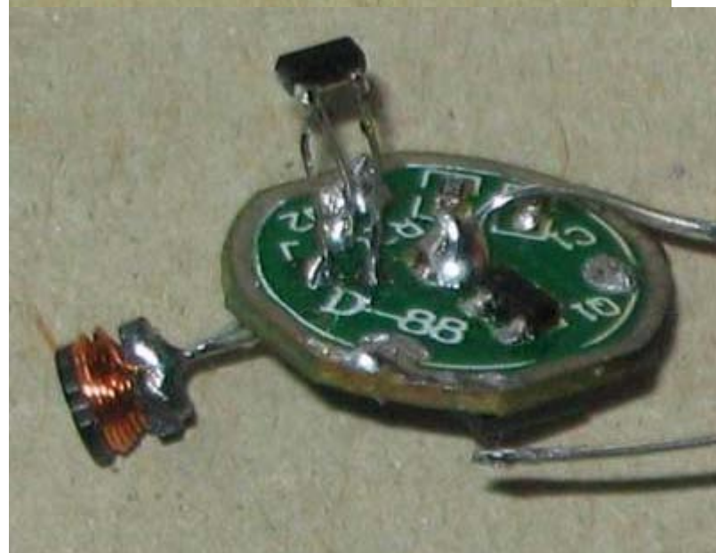
The controller has been placed on extension wires to test its operation.
