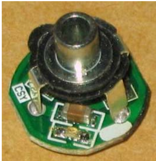
The LED and 1u capacitor can be clearly seen in this photo.
