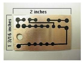
First, print out the PCB template to the left. From the left to the right of the PCB template...it should measure exactly two inches. From the bottom to the top of the PCB template...it should measure exactly 1- 3/16 inches. Send the picture to a graphics program, such as Paint, and squeeze and/or stretch to get a printout of the said dimensions. Once that is done, drill your hole for a SPST Sub-mini switch (Radio Shack part # 275-645A). Then mimmick the same routing as to the template.
