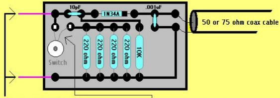
The two leads should be 1/2 inch long. Any gauge wire will suffice.
