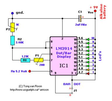
BUGFIX: Pin 3 error: Pin 3 goes to Vcc and point 'A'. Not pin 11 as previously indicated (Thanks Petr). I will redesign the circuit shortly and do away with the 1% resistors and the tantalum cap.
