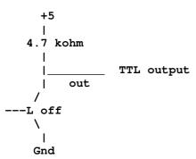
Therefore, an ECP/EPP pin can be set to "read mode" by setting it to 1, so the transistor pulling low is open (non-conducting) and the actual logical level on the pin can be read. This system is backward-compatible with SPP in most cases; some difficulties do arise, for example you can't get much power from the data pins.
