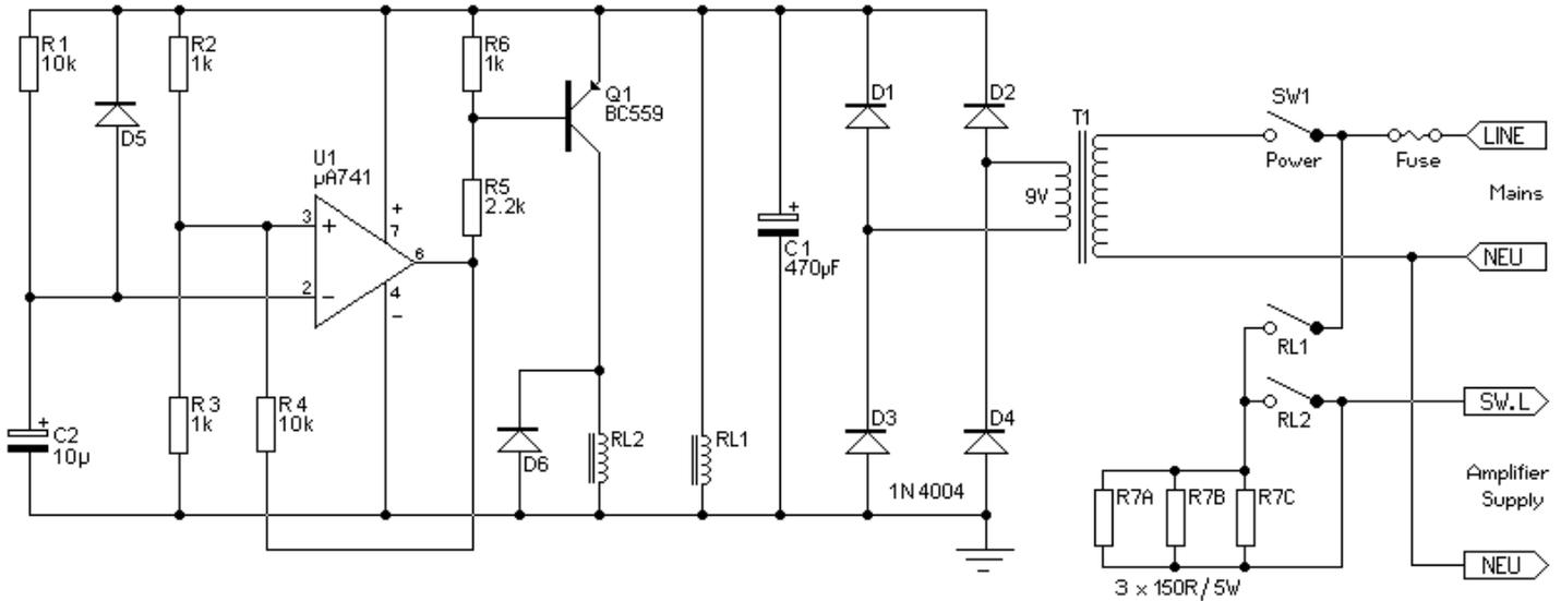
**Figure 6 - PCB Version of Soft Start/ Mains Switch**
