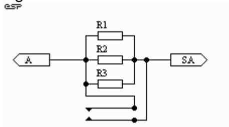
Figure 1 - Soft-Start Resistors and Relay Contacts
