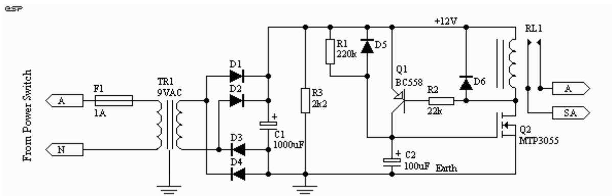
Figure 2 - Auxiliary Transformer Control Circuit
