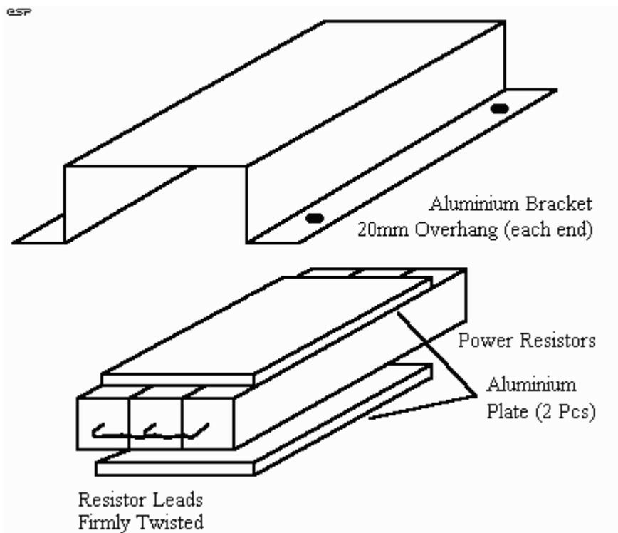
**Figure 5 - Suggested Resistor Mounting**
