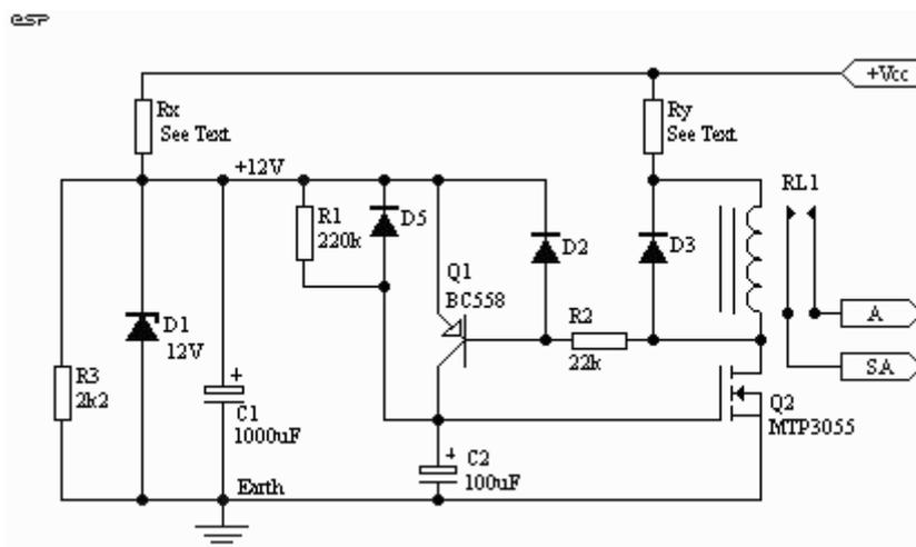
Figure 3 - Control Circuit Using Existing Supply
