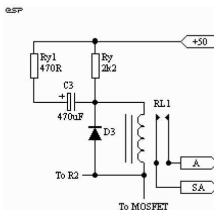
Figure 4 - Power Saving Relay Circuit
