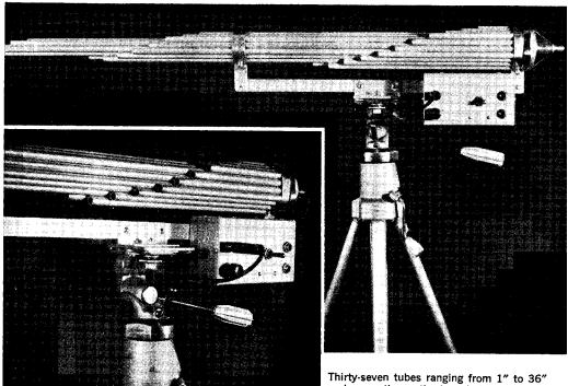
Thirty-seven tubes ranging from 1" to 36" make up the author's tubular mike; all construction details are given in text and in drawing at right. Completed unit is mounted on a camera tripod and panned like a machine gun to find sound source.
