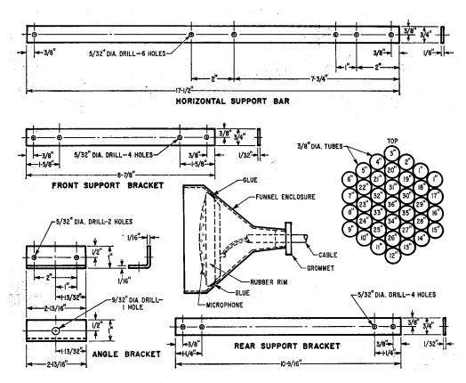
Easily worked aluminum is used for fabricating the pickup. The tubes can be conveniently cut from ten 6' lengths of 3/8" diameter stock, the support brackets from a sheet or strip of 1/32" aluminum. The horizontal support bar is made from heavier stock. Angle bracket mounts to standard camera tripod.
