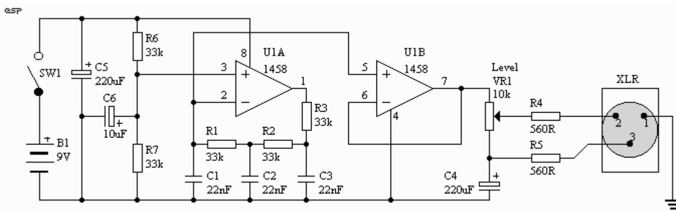
Figure 1 - Mic Circuit Test Oscillator
