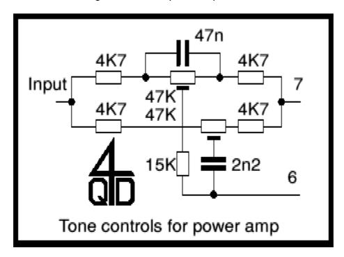
To use the tone controls you must break the link between 6 and 7 on the circuit. Also the 150K resistor, R13, should be decoupled. Replace it by two 68K resistors in series. The centre point of these two connects to the positive of a  $1\mu$  electrolytic whose negative connects to the earth (0v) line. This stops R13 acting as negative feedback which otherwise would shunt the tone controls.
