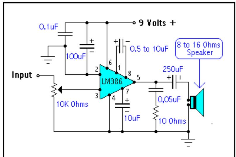
You can attach to the output of this circuit, speakers from 8 ohms to 16 ohms. I experimented with small speakers and even one of 7 inches in diameter showed excellent results!
