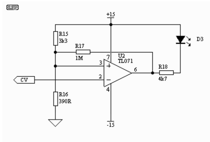
Figure 3 - Optional Schmitt Trigger Indicator
