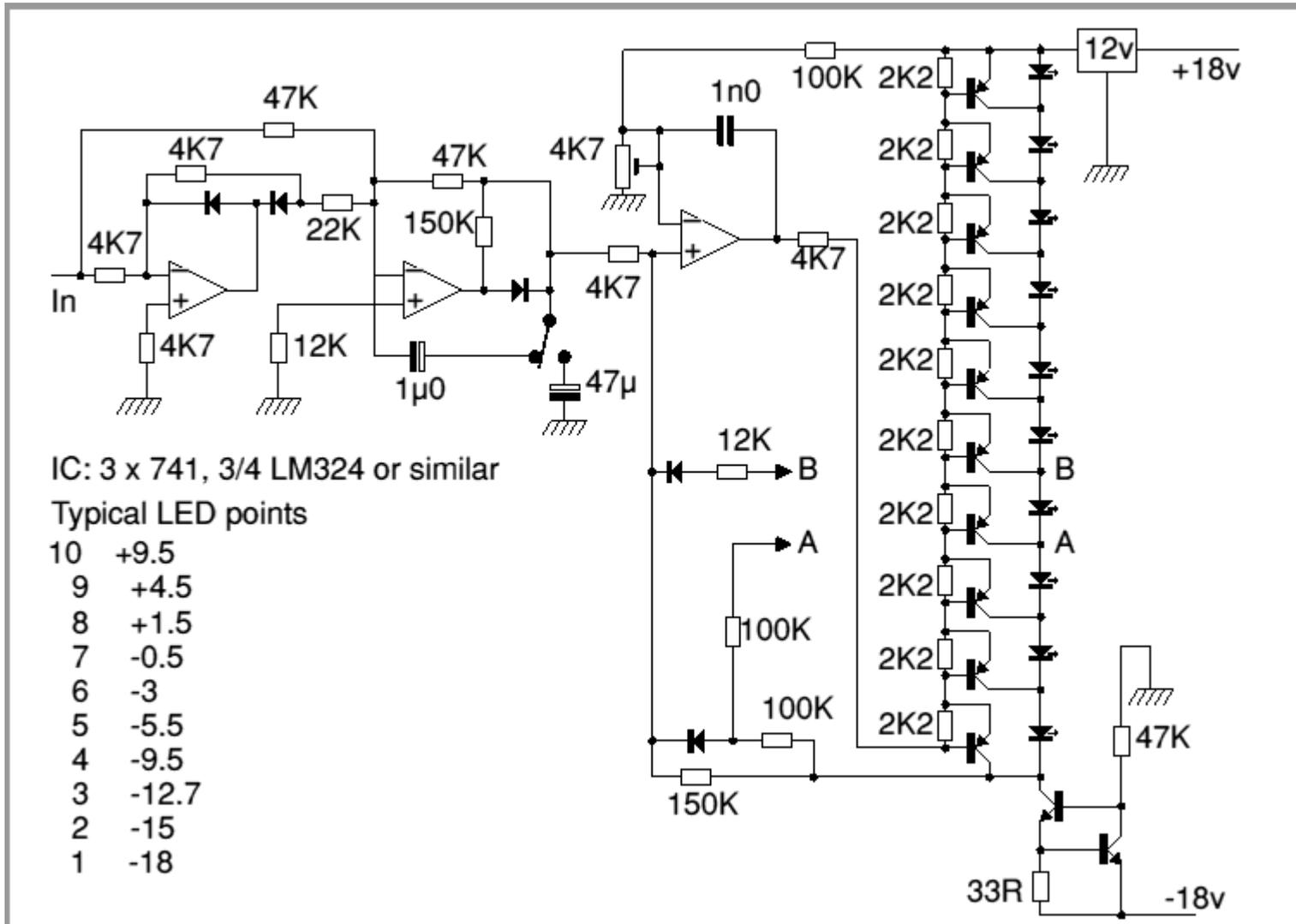
The circuit was designed to work with an audio power amplifier which operated off +18v-0v-18v power rails. The actual voltage used is not too critical except that the feedback is referred to the LED chain which itself is anchored to a +12v rail, hence the separate stabilizer for this. It has one large advantage over most of the LED chips available - all the LEDs are in series so it only draws 20mA irrespective of the number of LEDs illuminated.
