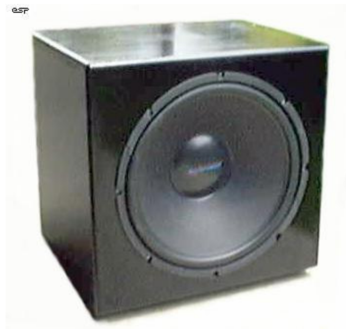
Figure 3 - Photo of Completed EAS Cabinet
